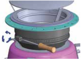
Figure 12aa3 Loosen the clamp on the sleeve rubber.
