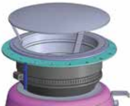
Figure 12aa4 Pull the sleeve upwards to separate it from the rubber
