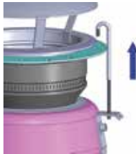
Figure12aa2 Pull the hooks up from the perforated sleeve to disconnect
